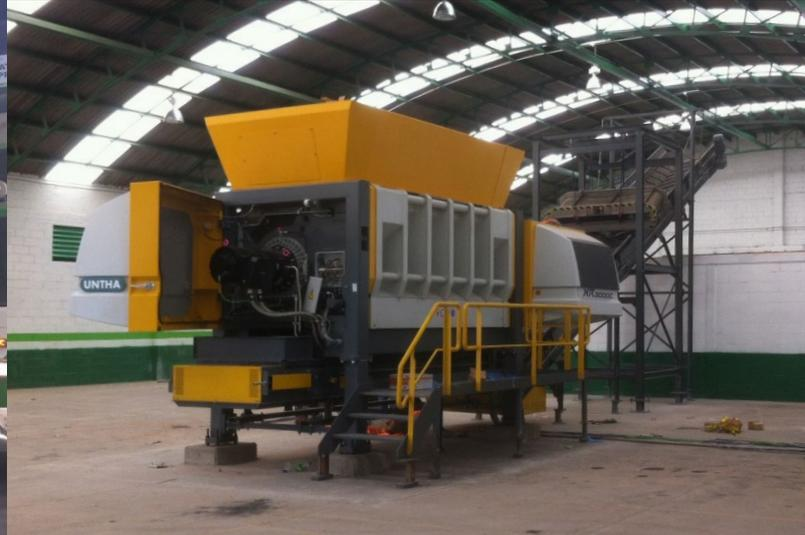
Following detailed discussions and trials, the XR was shipped to Mexico by sea-freight, complete with a discharge conveyor and overband magnet for metal extraction. During commissioning, the technology achieved the required output of 12 tonnes of processed feedstock per hour.
