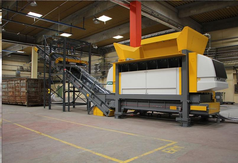
sensors, will automatically spray water onto the fire risk. If the risk is within the shredder, the materials can be cooled and/or the fire put out before anything is discharged from the machine. If the problem is on the conveyor, the nozzles prevent hot, glowing fractions from entering the pile of output material, where a fire could otherwise break out.
