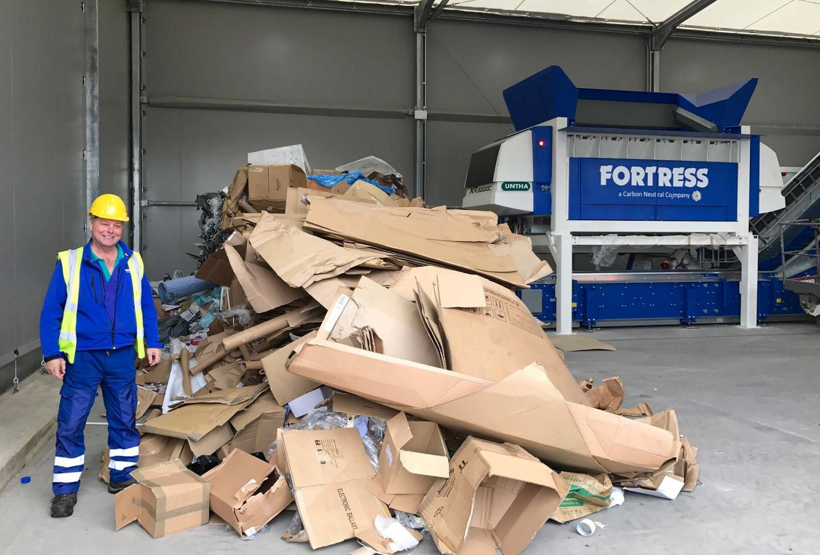
At present, the XR reduces the fraction to a homogenous 300mm particle size, but a simple cutting reconfiguration could achieve an output specification as low as 30mm.
