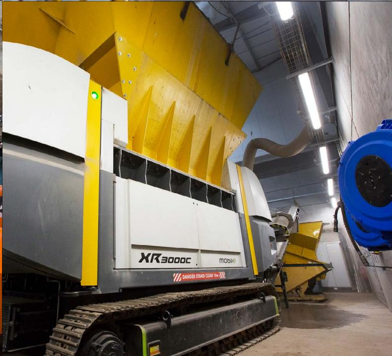
However, the XR's lower energy consumption has by far been the stand-out benefit for Rabbit to date. With its robust cutting concept, the machine is capable of processing various materials to further reduce the amount of complex waste sent for wider treatment or disposal, and the technology can be reconfigured to manufacture different fuel specifications in only three hours.
